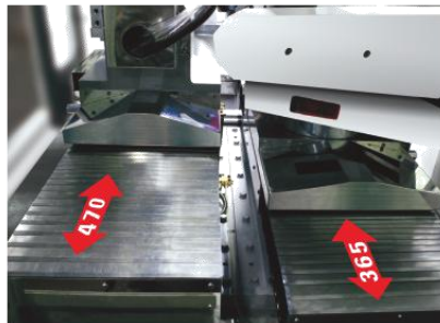
Internal grinding wheel workpiece stroke: 0~470 mm External grinding wheel workpiece stroke: 0~365 mm
